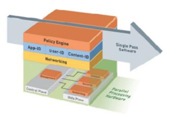
*App-ID*. Our application classification engine, called App-ID, uses multiple identification techniques to determine the exact identity of applications traversing the network. App-ID is the foundational classification engine that provides the core traffic classification to all other functions in our platform. The App-ID classification is used to invoke other security functions.
